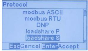
Select either "loadshare P" for the Primary ATevo, or "loadshare S" for a Secondary ATevo. Only one (1) ATevo can be the Primary. The other ATevo on the forced load sharing network must be set to Secondary.
