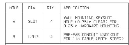
STANDARD PRE-FAB CONDUIT KNOCKOUTS ARE SHOWN. IF ADDITIONAL CONDUIT ENTRANCES ARE REQUIRED BY USER, ENCLOSURE SHOULD BE FIELD-MODIFIED BY INSTALLER.
