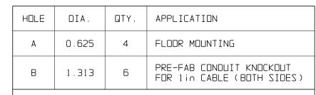
STANDARD PRE-FAB CONDUIT KNOCKOUTS ARE SHOWN. IF ADDITIONAL CONDUIT ENTRANCES ARE REQUIRED BY USER, ENCLOSURE SHOULD BE FIELD-MODIFIED BY INSTALLER.
