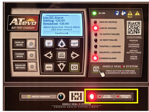
Figure 2B – Status LED for Action Required
